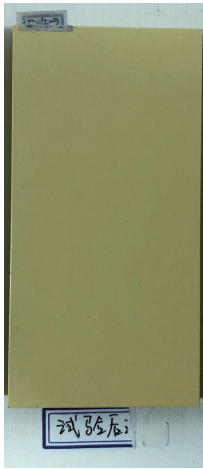
图6 PAA+BR-127+TB06-9腐蚀960h Fig.6 PAA+BR-127+TB06-9 after 960h corrosion
